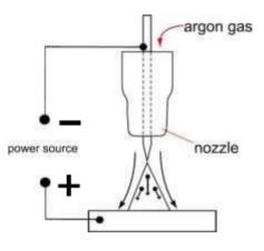
between the tungsten and the work piece is the TIG arc and can be as hot as 19,000°C. It is a very pure and concentrated arc which provides the controlled melting of most metals into a weld pool. TIG welding offers the user the greatest amount of flexibility to weld the widest range of material and thickness and types. DC TIG welding is also the cleanest weld with no sparks or spatter.
