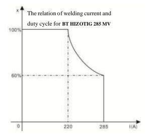
If the welding machine is overheating, the IGBT over-heat protection sensing will send a
