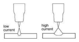
The intensity of the arc is proportional to the current that flows from the tungsten. The welder regulates the welding current to adjust the power of the arc. Typically thin material requires a less powerful arc with less heat to melt the material so
