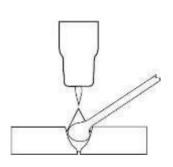
It is necessary in many situations with TIG welding to add a filler wire into the weld pool to build up weld reinforcement and create a strong weld. Once the arc is started the torch tungsten is held in place until a weld pool is created, a circular movement of the tungsten will assist is creating a weld pool of the desired size. Once the weld pool is established tilt the
