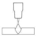
Manual TIG welding is often considered the most difficult of all the welding processes. Because the welder must maintain a short arc length, great care and skill are required to prevent contact between the electrode and the work piece. Similar to Oxygen Acetylene torch welding, TIG welding normally requires two hands and in most
