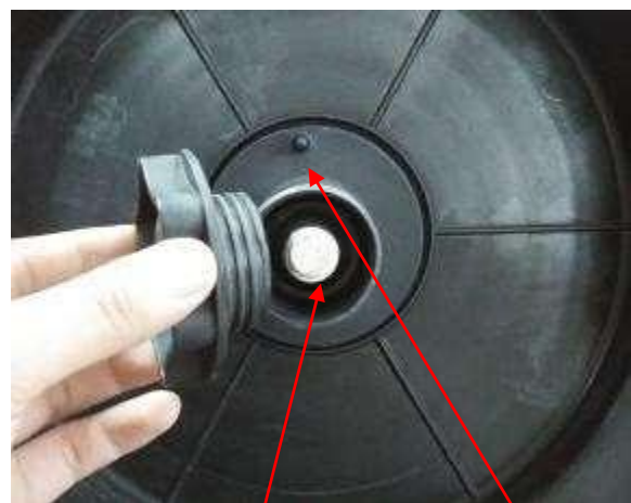
(2) Note the tension spring adjuster and spool locating pin.
