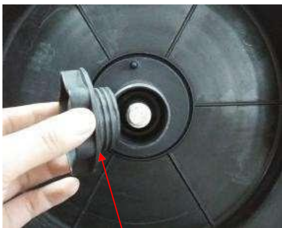
(1) Remove the spool retaining nut.
