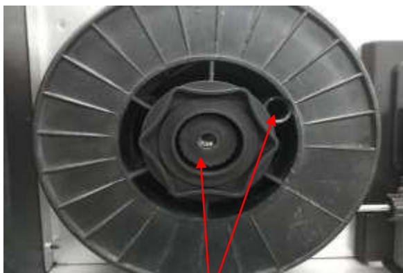
(3) Fit the wire spool onto the spool holder fitting the locating pin into the location hole on the spool. Replace the spool retaining nut tightly.
